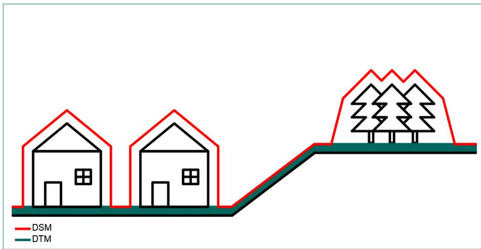
Figure 3-1 Difference between DSM and DTM – DEM
