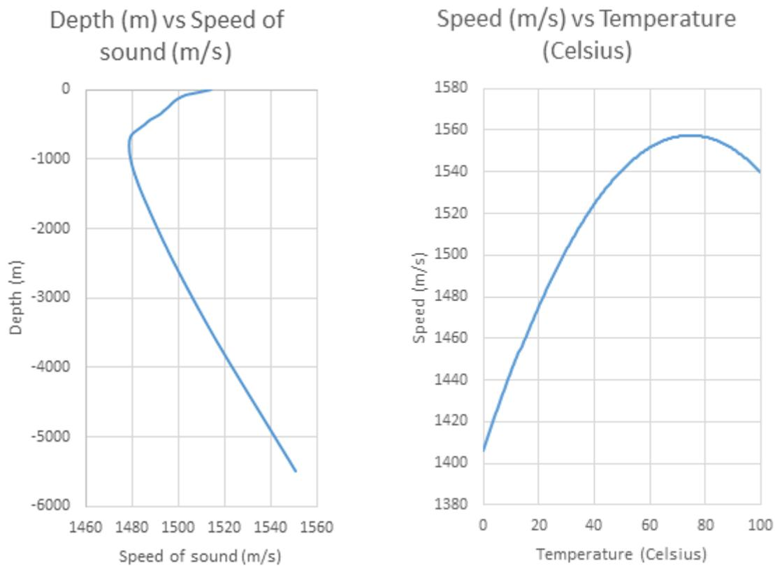
Figure 16-1 Sample of Sound Speed Variations at Different Depths and Temperatures
