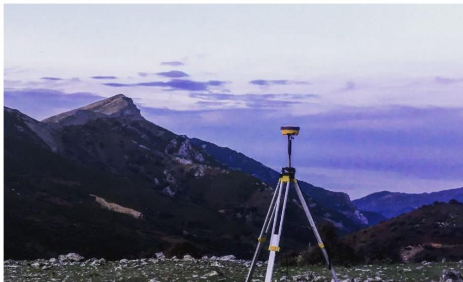
Figure 2-4 GNSS Base Station
