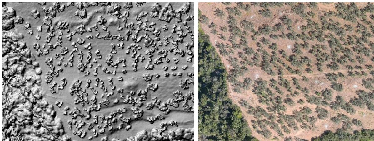
Figure 17-4 (a) Digital Surface Model from Photogrammetry and (b) Orthophotomosaic
