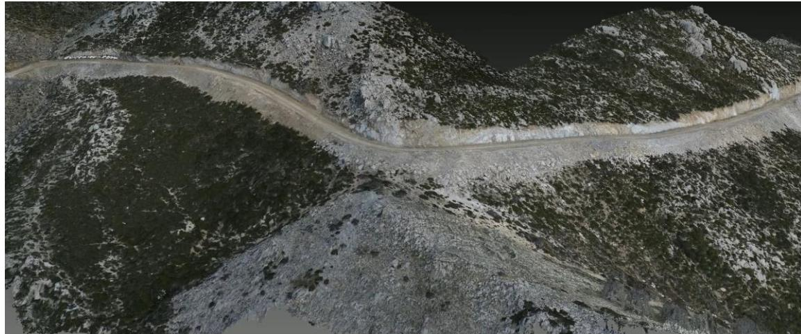
Figure 2-5 Aerial Survey Generated Point Cloud
