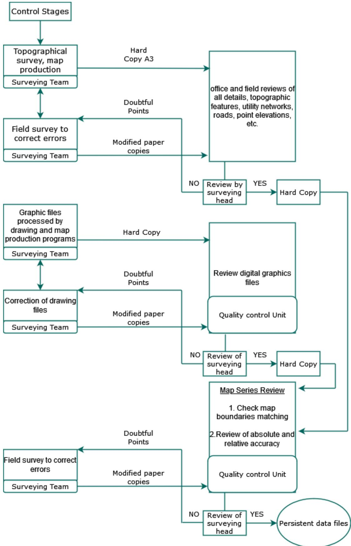
Figure 5-1 Flowchart for Quality Control of Topographic Maps (MoMRAH, 2005)
