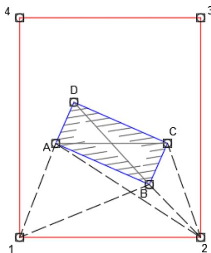
Figure 9-1 Intersection of Points by Distance Measurements Method
