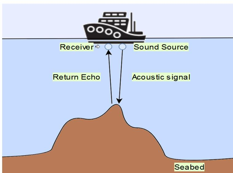
Figure 2-6 Illustration of Echo-Sounding Mechanism
