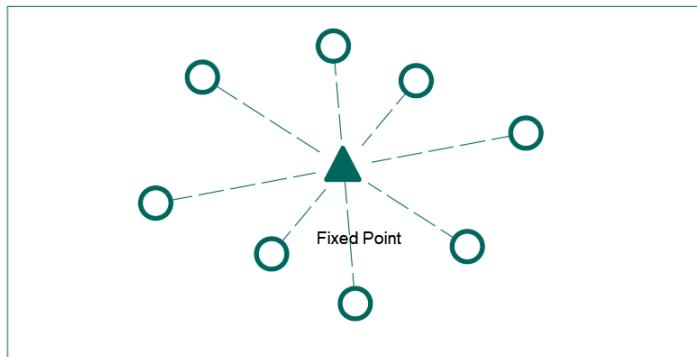
Figure 10-3 Fast Static Survey - Hollow Circles Represent Rovers
