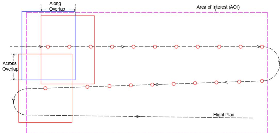
Figure 13-1 Typical Flight Pattern over Area of Interest
