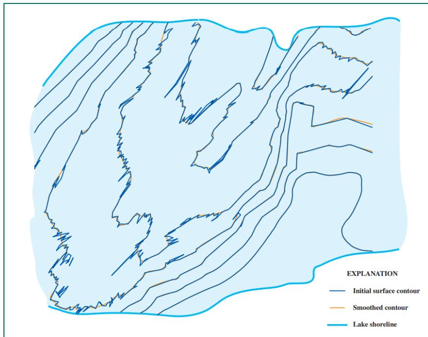
Figure 16-7 Representation of Initial Surface Contours and Cartographically Smoothed Contours (Wilson & Richards, 2006)
