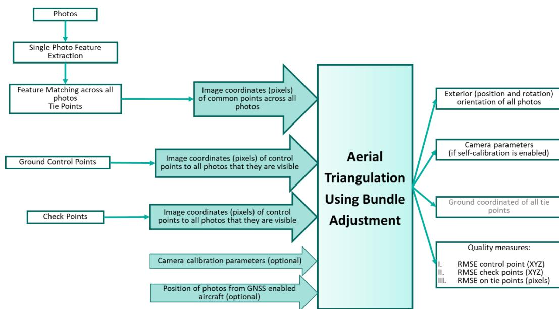
Figure 13-3 Aerial Triangulation Input and Output
