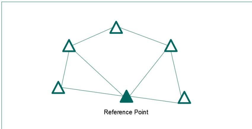
Figure 10-2 Static Survey - Hollow Triangles Represent Rovers
