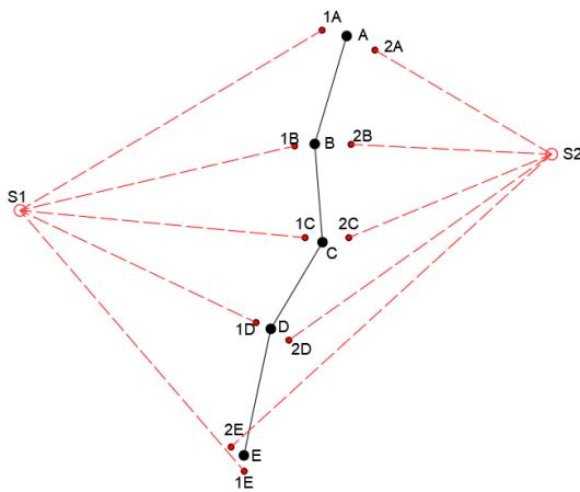
Figure 12-1 RTK Closure Error Analysis
