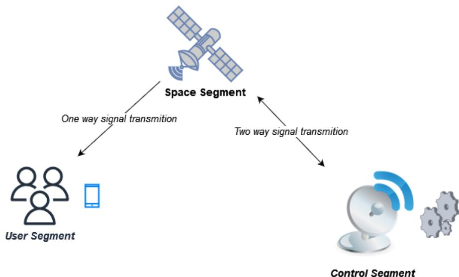
Figure 10-1 GNSS Components
