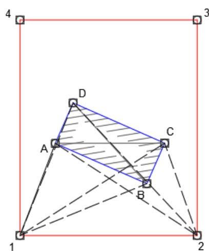
Figure 9-6 Intersection of Points by Angle Measurements Method
