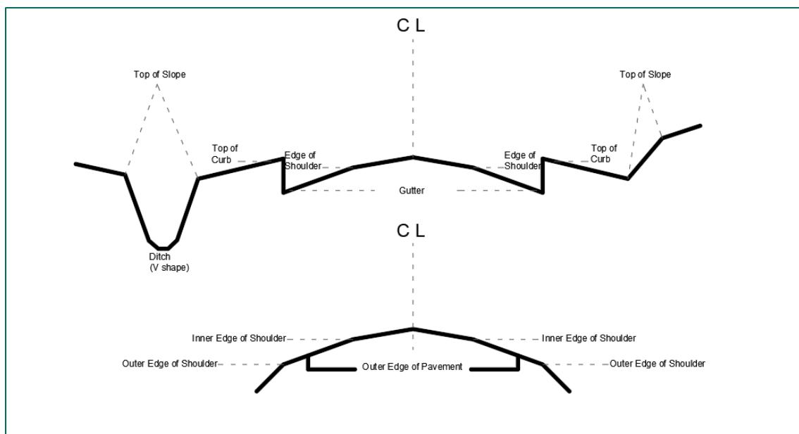
Figure 17-3 Breaklines Placement - Typical Section
