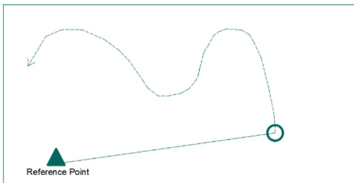
Figure 10-5 Kinematic Survey - Hollow Circle Represent Rover Positions
