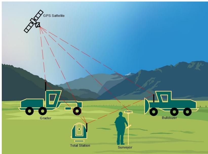
Figure 19-2 Equipment for AMG Methods
