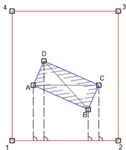
Figure 9-3 Orthogonal Method
