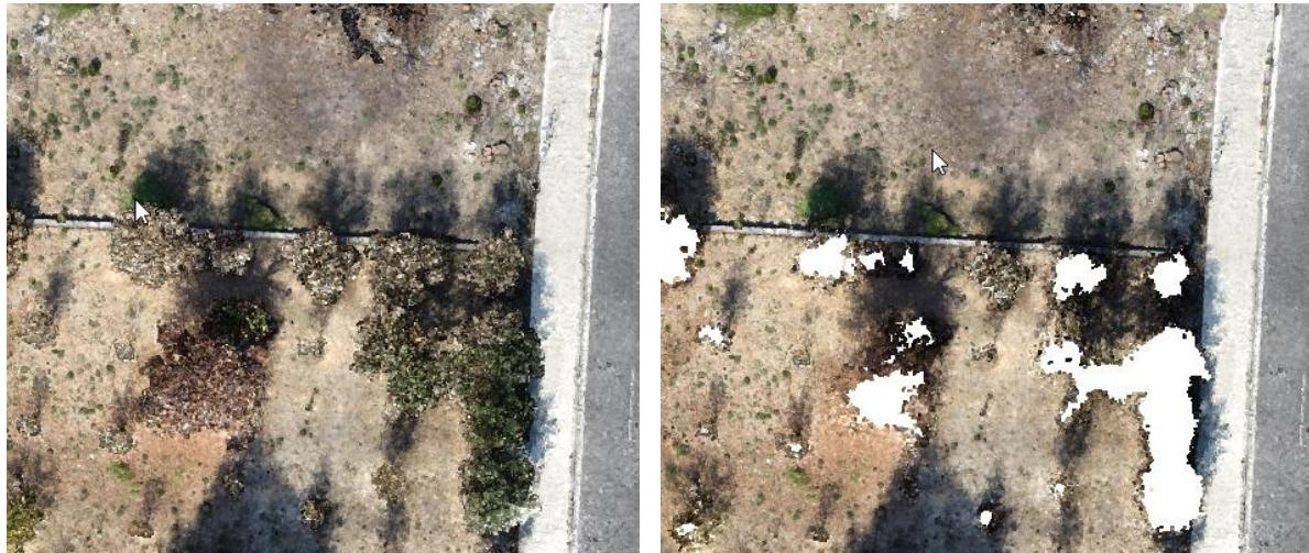
Figure 17-5 (a) Raw Point Cloud and (b) Automatically Identified Ground Point Cloud Data
