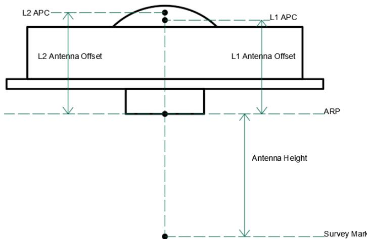
Figure 11-1 Antenna Reference Point (ARP) and Antenna Phase Center (APC) for L1 and L2 and Offsets
