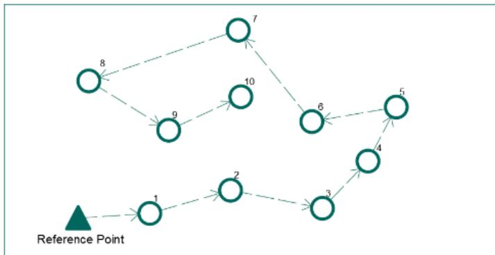
Figure 10-4 Stop-and-Go Kinematic Survey - Hollow Circles Represent Rover Positions
