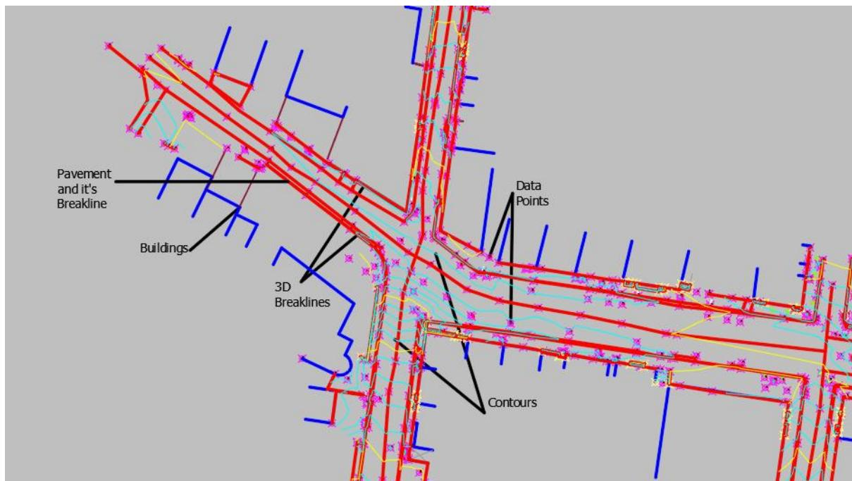
Figure 17-1 Typical DTM Features Collection
