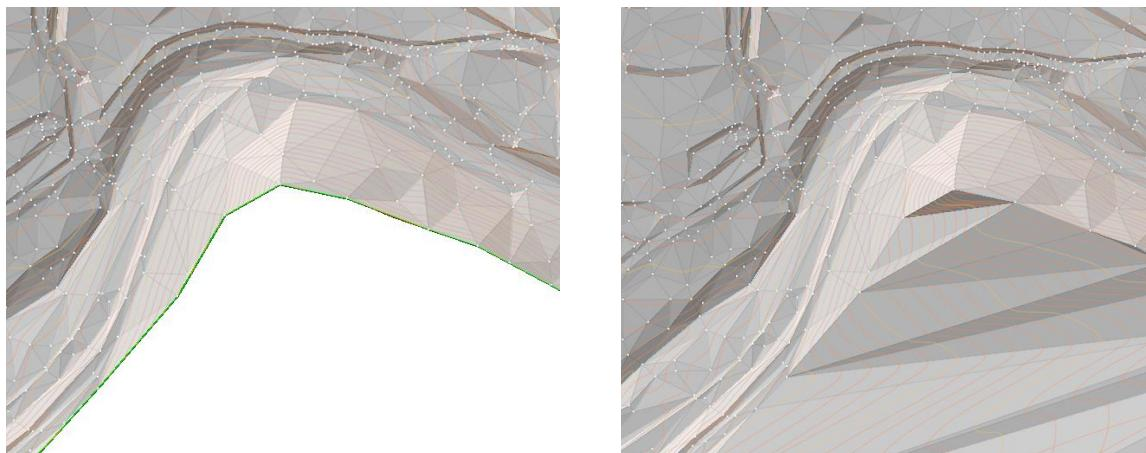
Figure 17-6 DTM Creation (a) With Outer Boundary and (b) Without Outer Boundary
